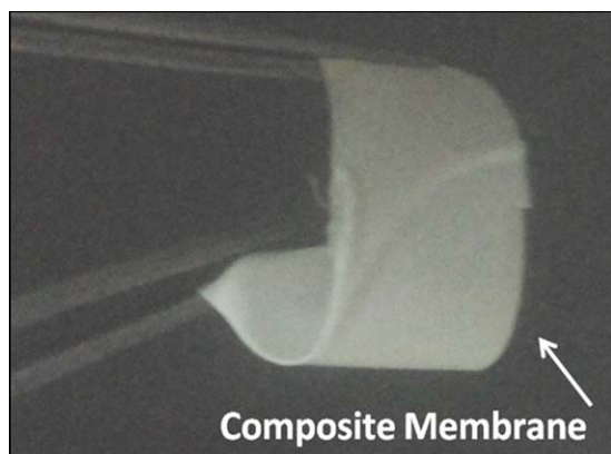
Figure 3. A digital image showing the nanocomposite-based flexible membrane.
